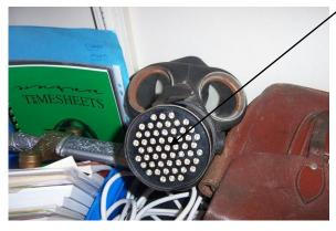
$\frac{\text{Store } 25}{\text{be an ACM}}$  – gas mask filter is presumed to be an ACM. Removal is recommended as soon as possible
