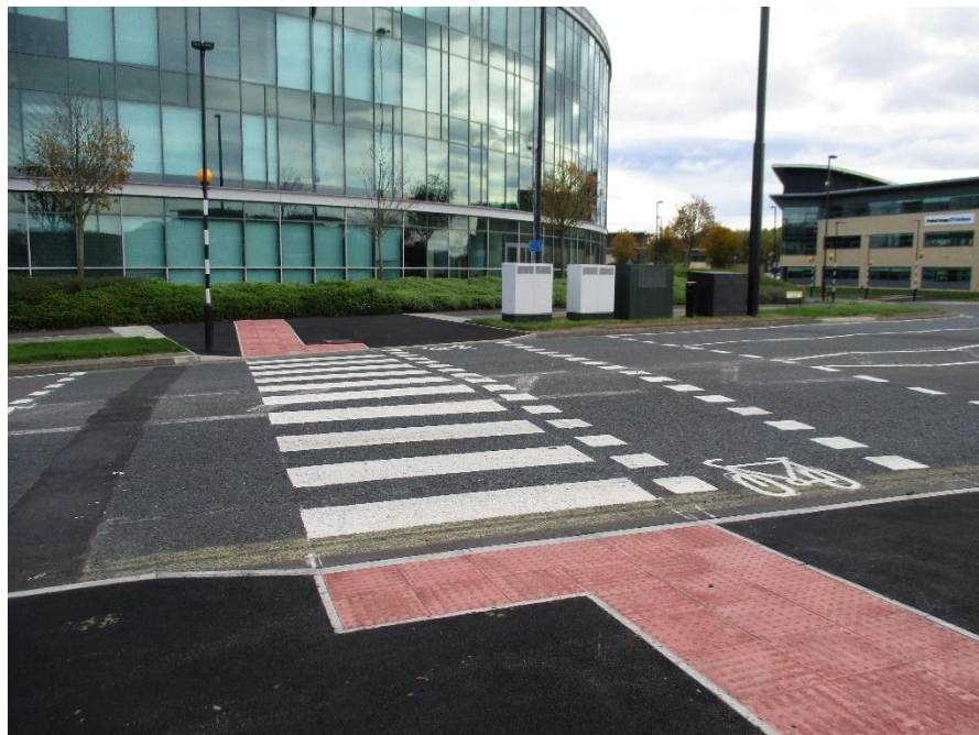
Photo 23 - Example of Parallel Crossing at Roundabout in Cobalt Business Park, North Tyneside
