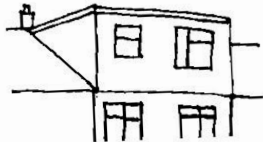
A top heavy design appears overly dominant in the street scene and is detrimental to the property.
