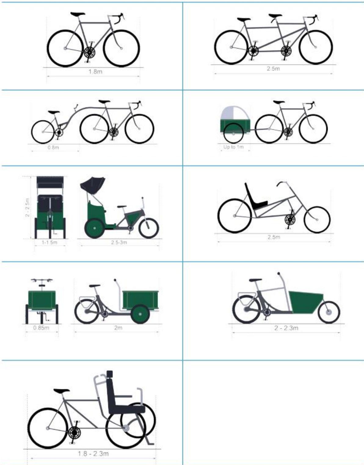
Figure 3 - Typical forms of cycles and their dimensions (LTN1/20)
