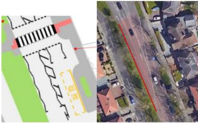
Figure 1-4 – Bus stop proximity to proposed crossing
