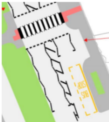
Figure 1-6 – Crossing protruding over driveway, A193 Broadway roundabout southern arm (east side).
