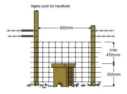
NB. If the fencing is higher, the stile will require an additional step (please refer to drawings of standard stiles for the dimensions of two-step stiles).
